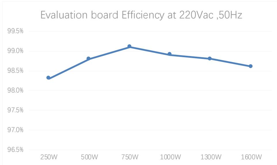
Figure 2. Efficiency at 220V input.
